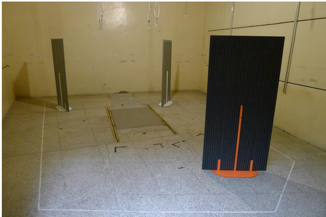
Fig. 1. View of the sample in reverberation chamber
